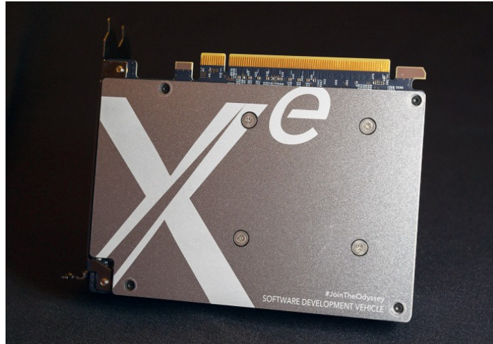
Figure 4.8 Intel's Xe DG1 GPU in Yarrow
